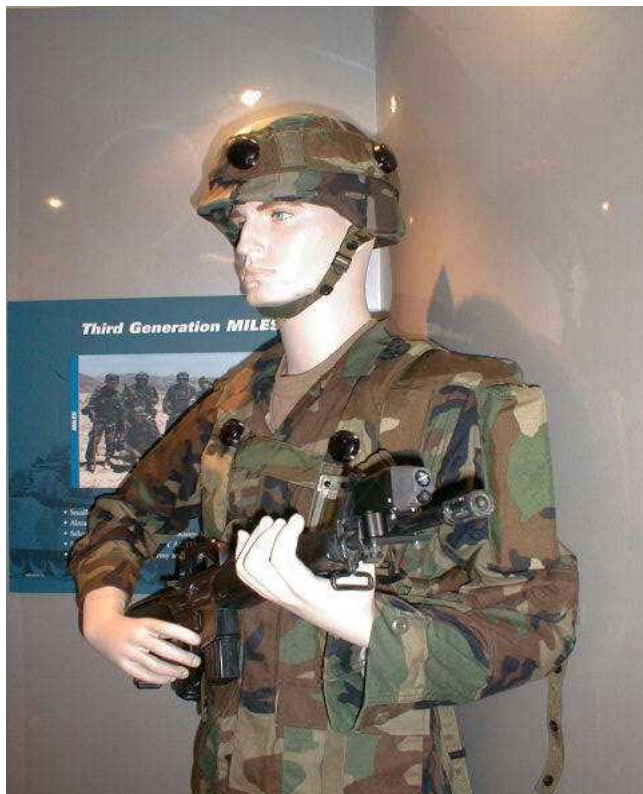
Figure 3: Laser generator mounted on rifle and detectors.
