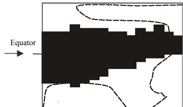
Figure 6: Illustration of results from cleaning trails with reduced cleaning time compared to the standard EHEDG test method. Black is uncleaned zones. Dotted lines mark the zones predicted as cleanable from a critical wall shear stress of 2.5 - 3 \text{ Pa} .
