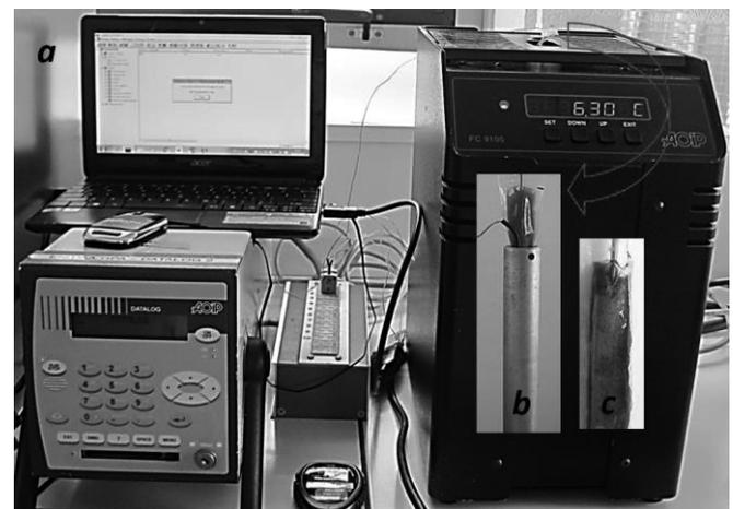
Figure 1. (a) experimental apparatus (b) heating vessel and in-package sample (c) sample packed in pouch.
