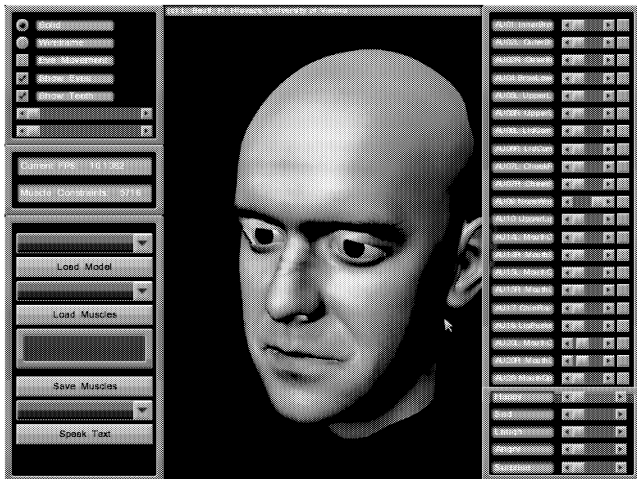
Figure 7: Simulation with Action Unit 9 (Nose Wrinkler) and 20 (Lip Corner Puller) activated
