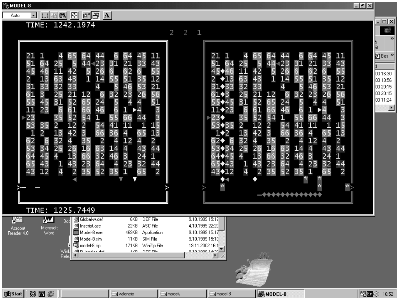
Figure 2: Reflective Simulation of a Container Yard – on the Left There is Animation of the External Model and on the Right There is Animation of the Internal Model. In it the Computer Controlling the Yard is Just Testing Whether two Paths (Represented by Trapezoids) Will not Come to a Conflict.
