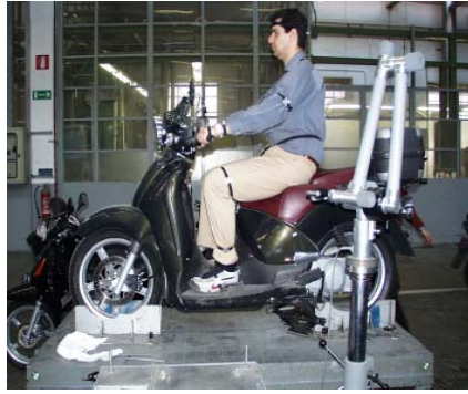
Figure 7. Experimental set-up for measurement of motorcycle posture.
